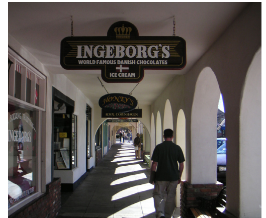
Hanging signs must maintain eight feet of clearance between the bottom of the sign and ground level
